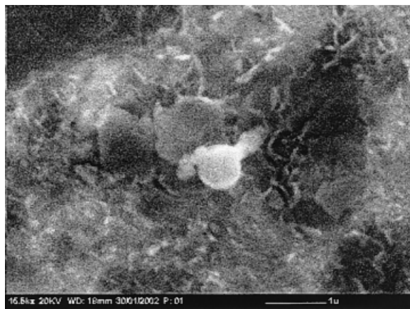
Figure 5. Zinc surface morphology after cathodic polarisation in containing ZAPP solution.
